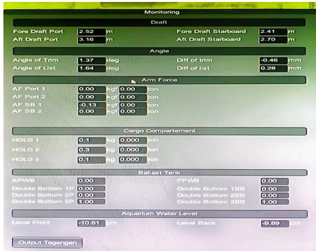
Figure 31. Data Monitoring Draft, Angle, Arm Force, Cargo Compartment, and Aquarium Water Level (c)
