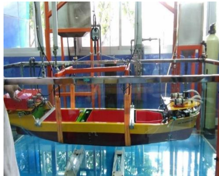
Figure 13. Installation Hoist is a tool to lift and weigh the ship before being floated
