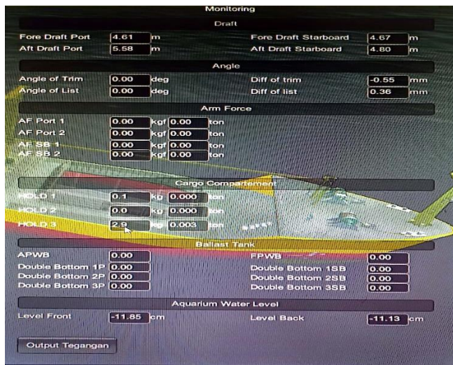
Figure 30. Data Monitoring Draft, Angle, Arm Force, Cargo Compartment, and Aquarium Water Level (b)
