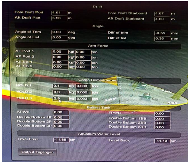
Figure 29. Data Monitoring Draft, Angle, Arm Force, Cargo Compartment and Aquarium Water Level (a)
