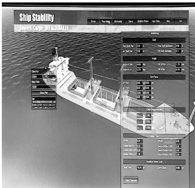
Figure 32. Data Monitoring Draft, Angle, Arm Force, Cargo Compartment and Aquarium Water Level (d)
